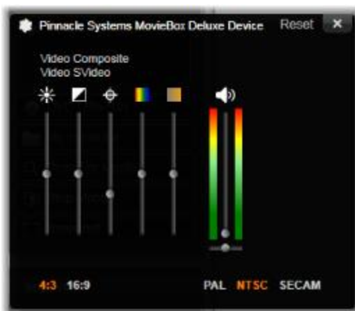
The Input Levels window lets you adjust a number of video and audio parameters. The Hue slider (fourth from left) is not used with PAL sources.
