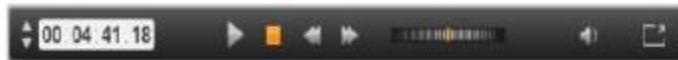
The transport bar for DV and HDV import, with (from left) jog controls and timecode readout, transport buttons, a shuttle control, and an audio button with a pop-out slider for controlling the preview volume.
