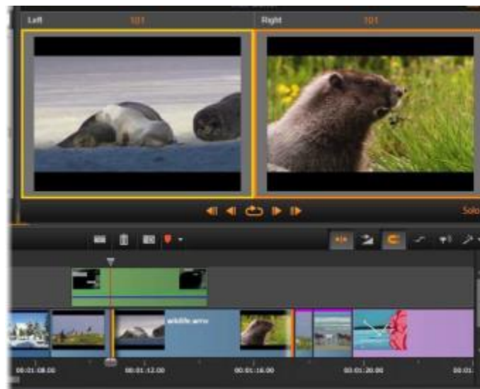
The Trim Editor in a slip trim operation. The left preview shows the currently selected trim point; the right preview shows the second trim point.
