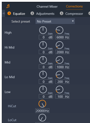
The controls for the Equalize correction feature. The dials let you set Gain and Frequency and the HiCut and LoCut settings.
